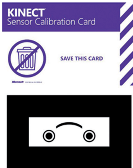
Figure 4. Kinect calibration card. To recalibrate the Kinect sensor, the RGB camera's coordinate system determines the 3D coordinates of the feature points on the calibration card, which are considered to be the true values.
