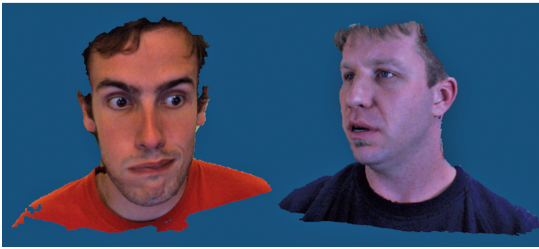
Figure 11. A screen shot of two remote people viewed from a third location. An enhanced 3D capture device runs in real time with multiple infrared (IR) projectors, IR cameras, and RGB cameras.
